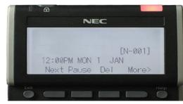
Press the soft touch key Del to delete the massage, other options like rewind / Re-direct / Call / Replay / Fast Forward are found under the More Soft touch key
